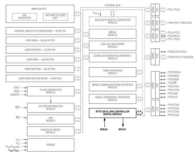
Figure 4-1. Block Diagram Highlighting BLDC Block and Pins
