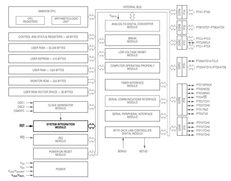
Figure 13-1. Block Diagram Highlighting SIM Block and Pins
