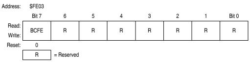
Figure 13-20. SIM Break Flag Control Register (SBFCR)
