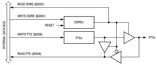
Figure 11-16. Port E I/O Circuit
