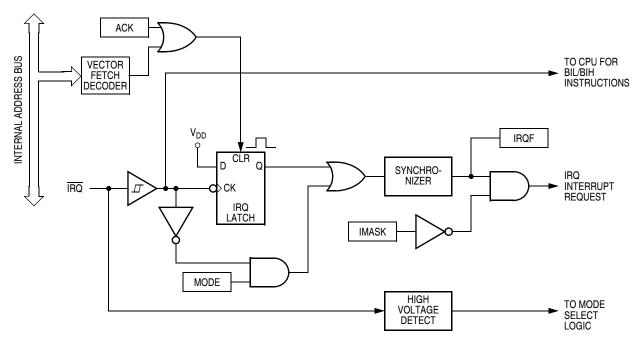
Figure 8-1. IRQ Block Diagram
