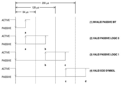
Figure 4-9. J1850 VPW Received Passive Symbol Times
