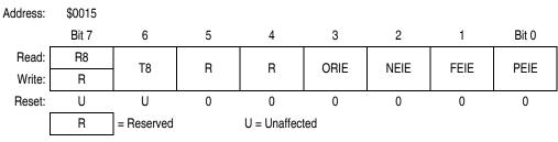
Figure 12-10. SCI Control Register 3 (SCC3)
