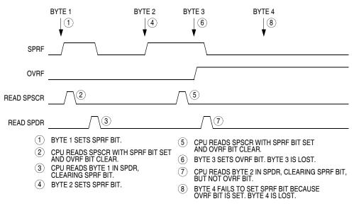
Figure 14-9. Missed Read of Overflow Condition
