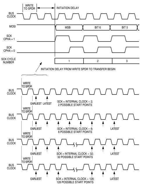
Figure 14-8. Transmission Start Delay (Master)
