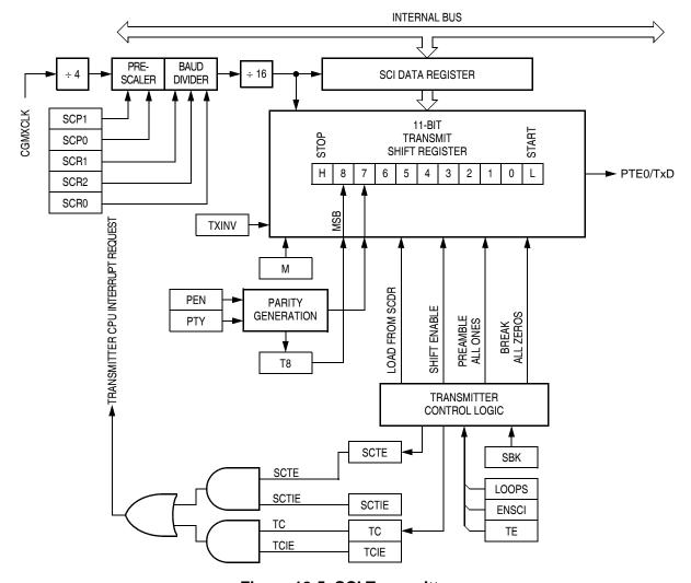
Figure 12-5. SCI Transmitter
