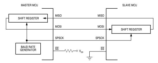
Figure 14-4. Full-Duplex Master-Slave Connections
