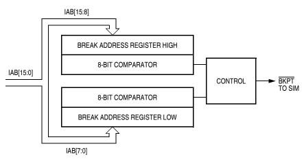
Figure 16-1. Break Module Block Diagram
