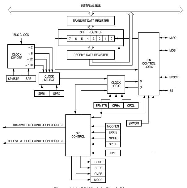
Figure 14-2. SPI Module Block Diagram
