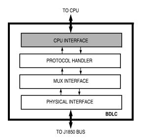
Figure 4-16. BDLC Block Diagram
