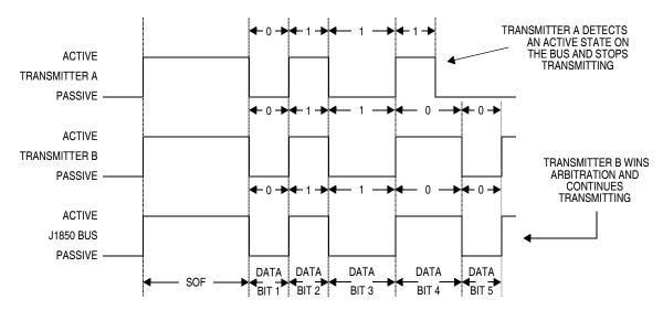
Figure 4-13. J1850 VPW Bitwise Arbitrations
