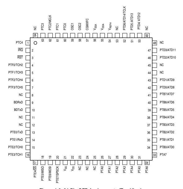
Figure 1-3. 64-Pin QFP Assignments (Top View)
