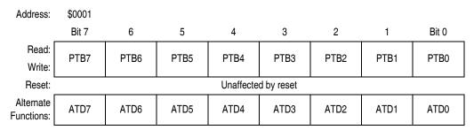
Figure 11-5. Port B Data Register (PTB)
