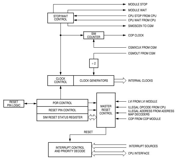
Figure 13-2. SIM Block Diagram
