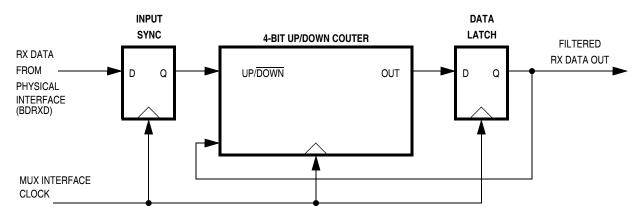
Figure 4-6. BDLC Rx Digital Filter Block Diagram
