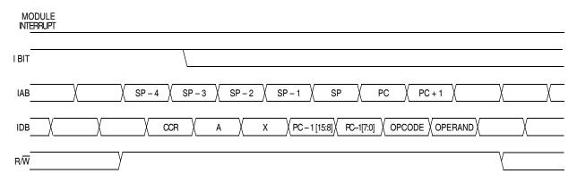
Figure 13-10. Hardware Interrupt Recovery
