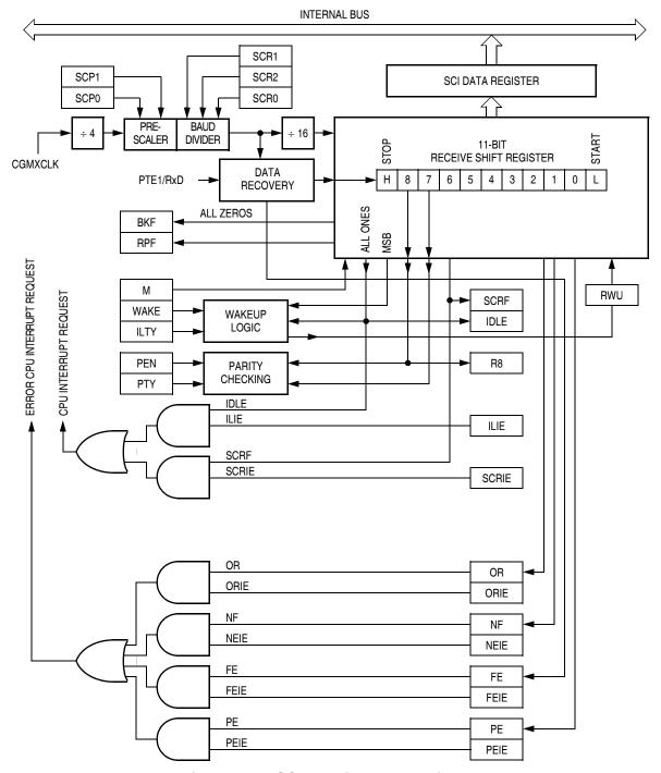
Figure 12-6. SCI Receiver Block Diagram
