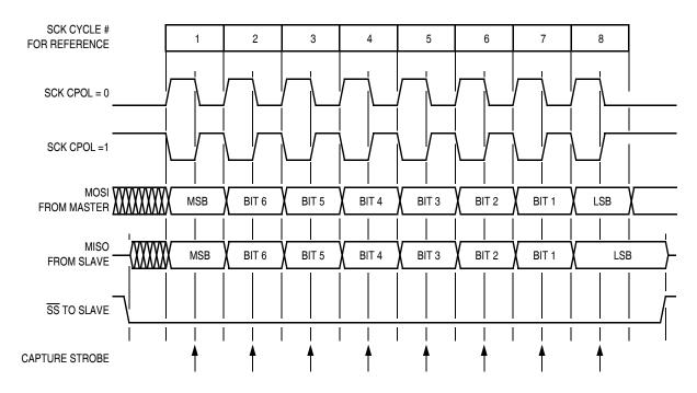
Figure 14-7. Transmission Format (CPHA = 1)
