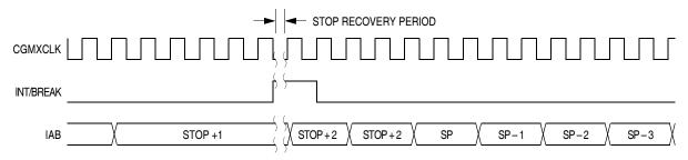
Figure 13-17. Stop Mode Recovery from Interrupt or Break
