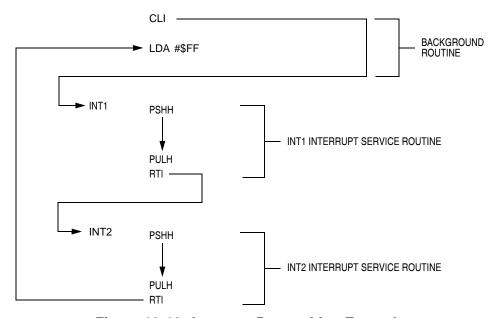
Figure 13-12. Interrupt Recognition Example
