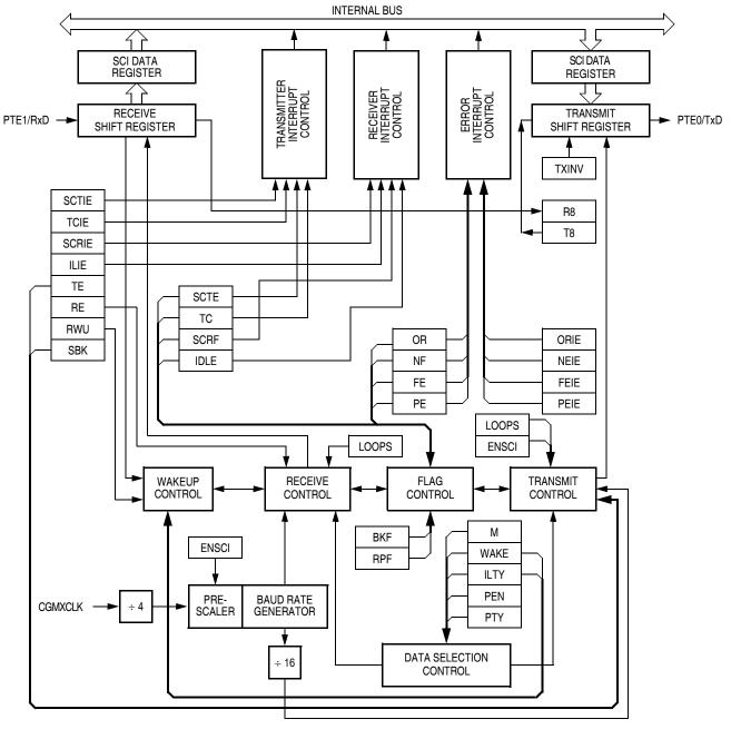
Figure 12-3. SCI Module Block Diagram
