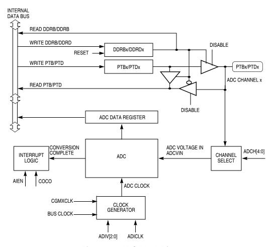
Figure 3-2. ADC Block Diagram
