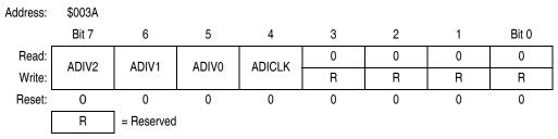
Figure 3-5. ADC Input Clock Register (ADICLK)
