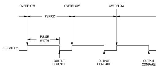
Figure 15-4. PWM Period and Pulse Width
