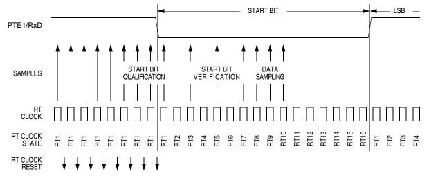
Figure 12-7. Receiver Data Sampling
