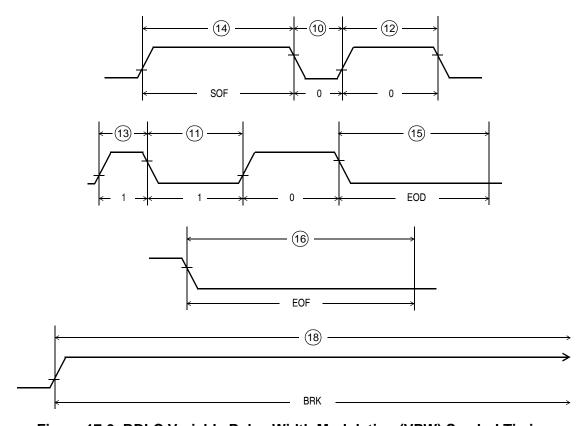
Figure 17-3. BDLC Variable Pulse Width Modulation (VPW) Symbol Timing
