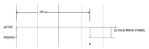
Figure 4-12. J1850 VPW Received BREAK Symbol Times
