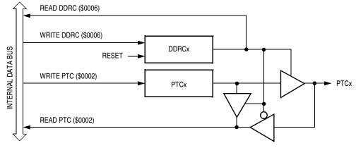
Figure 11-10. Port C I/O Circuit
