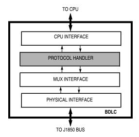
Figure 4-14. BDLC Block Diagram
