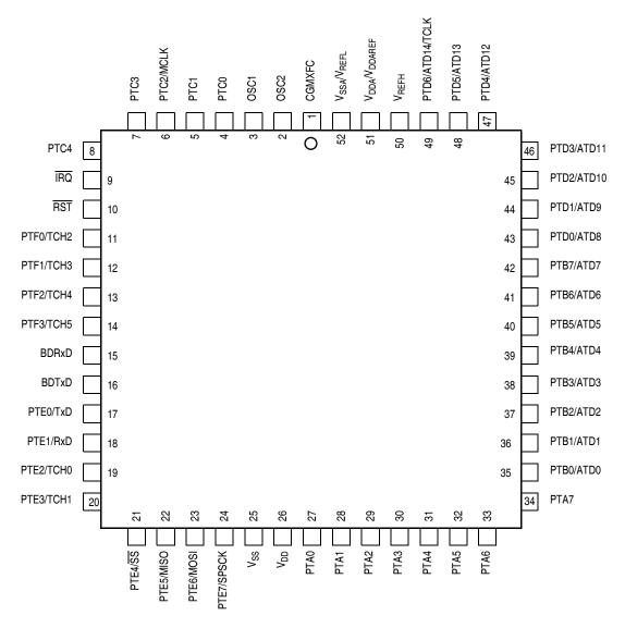
Figure 1-2. 52-Pin PLCC Assignments (Top View)
