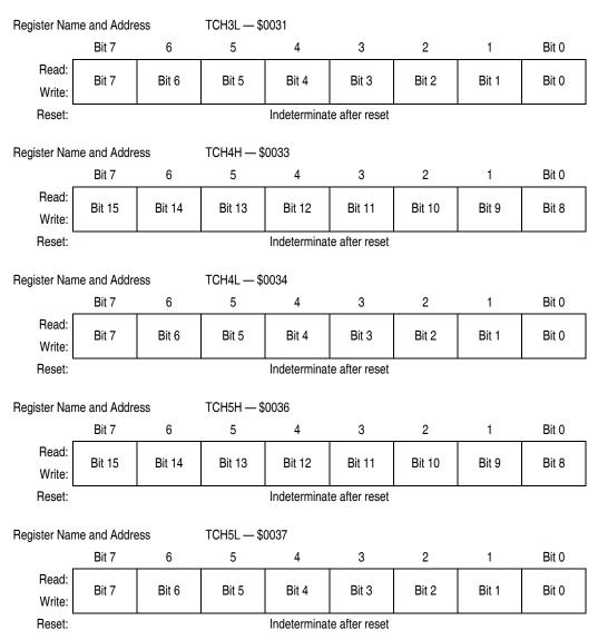
Figure 15-10. TIM Channel Registers (TCH0H/L-TCH3H/L) (Sheet 2 of 2)
