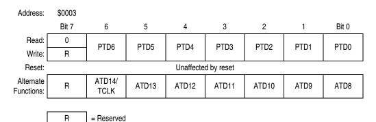
Figure 11-11. Port D Data Register (PTD)
