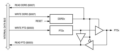
Figure 11-13. Port D I/O Circuit
