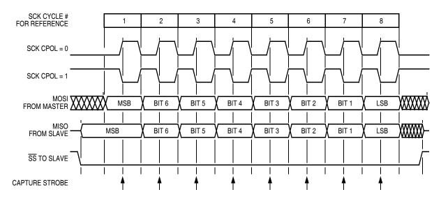
Figure 14-5. Transmission Format (CPHA = 0)
