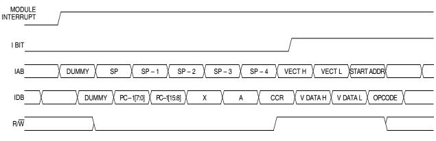
Figure 13-9. Hardware Interrupt Entry
