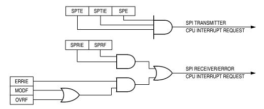
Figure 14-11. SPI Interrupt Request Generation
