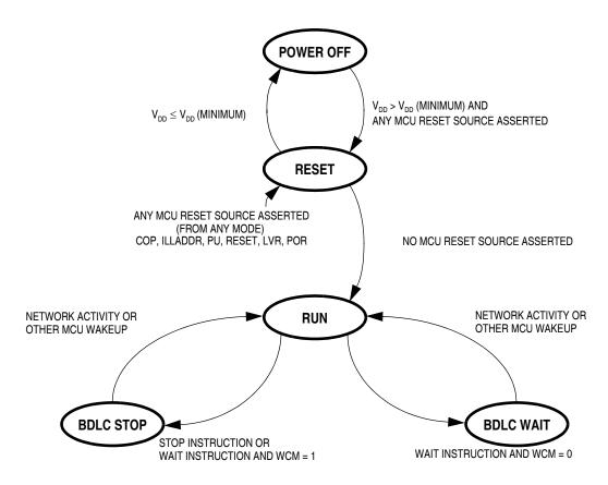
Figure 4-4. BDLC Operating Modes State Diagram
