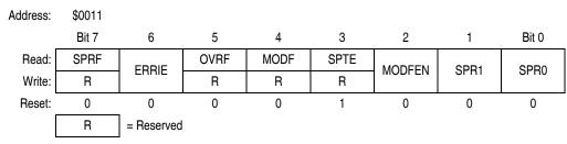
Figure 14-15. SPI Status and Control Register (SPSCR)
