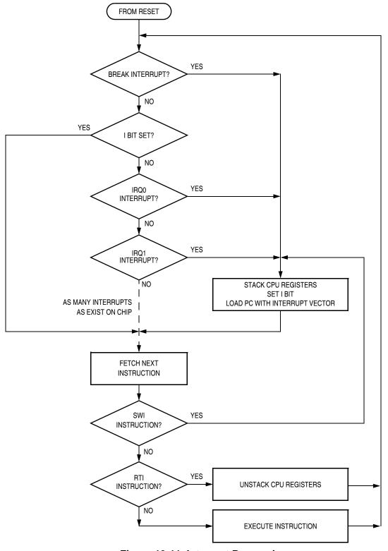
Figure 13-11. Interrupt Processing
