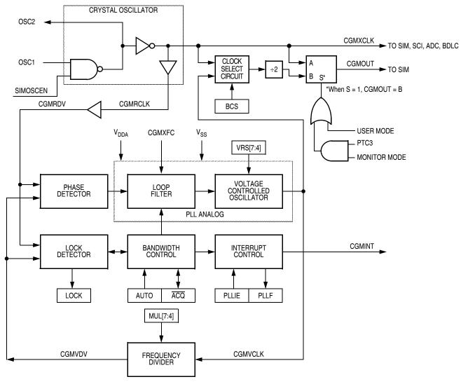
Figure 5-1. CGM Block Diagram
