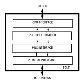
Figure 4-2. BDLC Block Diagram
