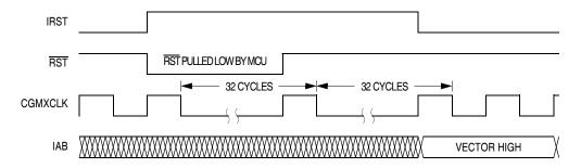
Figure 13-6. Internal Reset Timing
