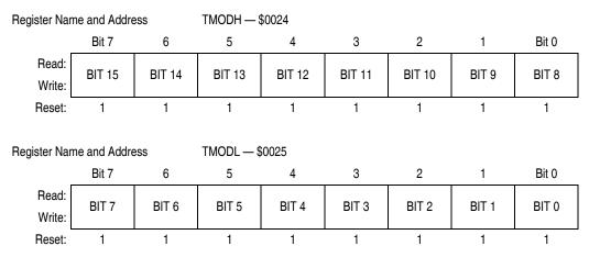
Figure 15-7. TIM Counter Modulo Registers (TMODH and TMODL)
