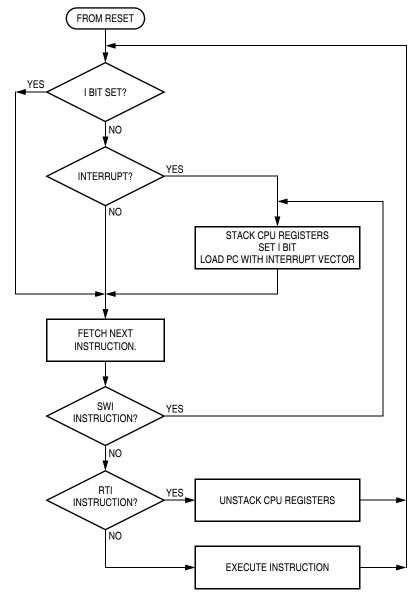
Figure 8-4. IRQ Interrupt Flowchart
