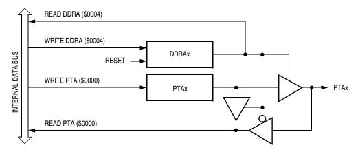
Figure 11-4. Port A I/O Circuit
