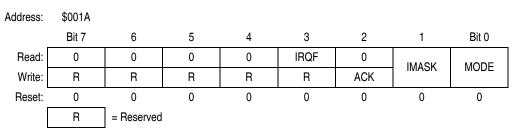
Figure 8-5. IRQ Status and Control Register (ISCR)
