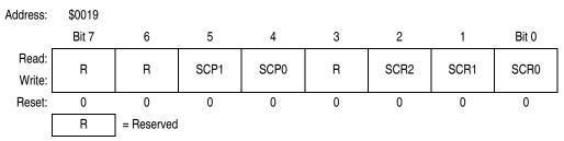
Figure 12-15. SCI BAUD Rate Register (SCBR)
