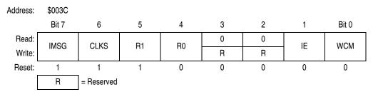
Figure 4-18. BDLC Control Register 1 (BCR1)
