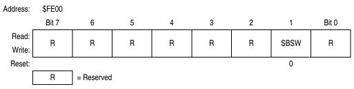
Figure 13-18. SIM Break Status Register (SBSR)
