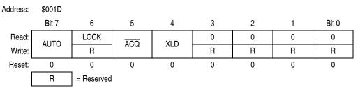
Figure 5-5. PLL Bandwidth Control Register (PBWC)
