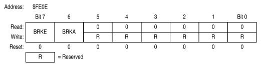
Figure 16-3. Break Status and Control Register (BRKSCR)
