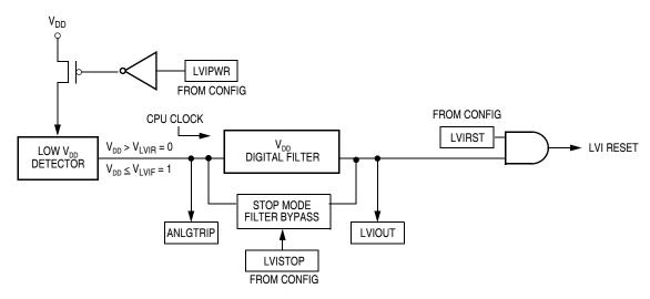
Figure 9-1. LVI Module Block Diagram
