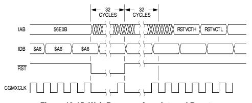
Figure 13-15. Wait Recovery from Internal Reset
