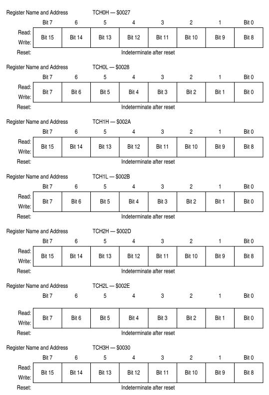
Figure 15-10. TIM Channel Registers (TCH0H/L-TCH3H/L) (Sheet 1 of 2)
