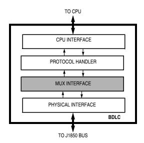
Figure 4-5. BDLC Block Diagram
