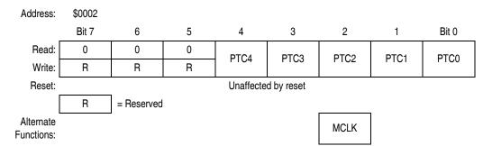
Figure 11-8. Port C Data Register (PTC)
